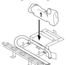
Figure 53 - Installing Log No. 1
